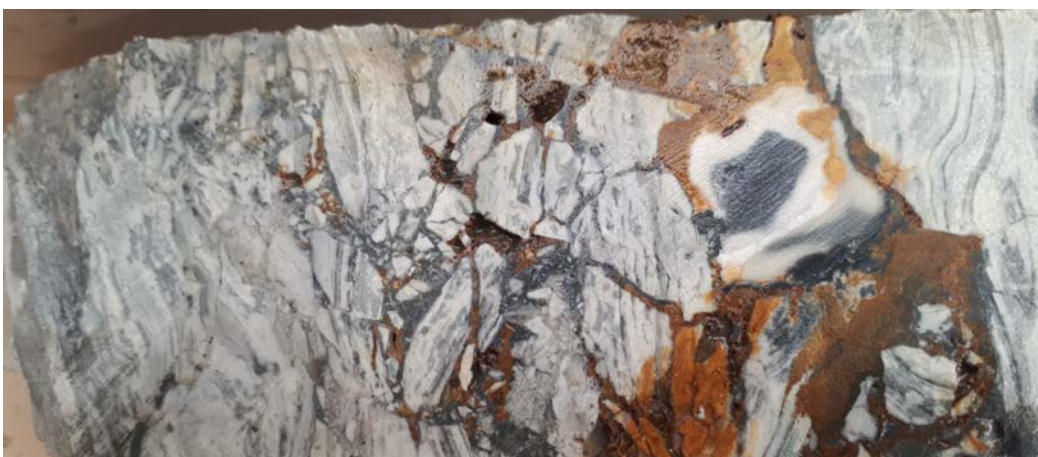
CAL18-12 – 21m downhole. Sample of oxidized breccia, sample interval (20.5-21.3m) assayed 14.3 g/t Au + 35 g/t Ag.
